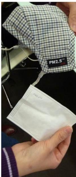
**Photo 3** This device, whilst it looks good, claims to meet filter 97.5% of fine particles. It uses a replaceable filter. Most of the air breathed in will not pass through the filter. It cannot work effectively
